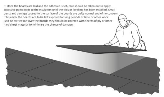
7: It is advisable to fit the final floor covering as soon as possible once the insulation has been installed. When fitting the chosen final floor covering it is advisable to work on top of a hard board. This will help prevent damage to the insulation when the work is being carried out.
