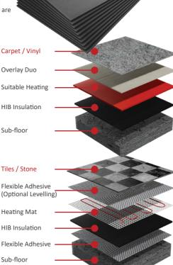
1: The sub-floor, whether concrete or wood, should be made suitable for the chosen floor covering (ie tiles) prior to any boards being fitted. The boards are designed to provide increased insulation levels not structural rigidity.
